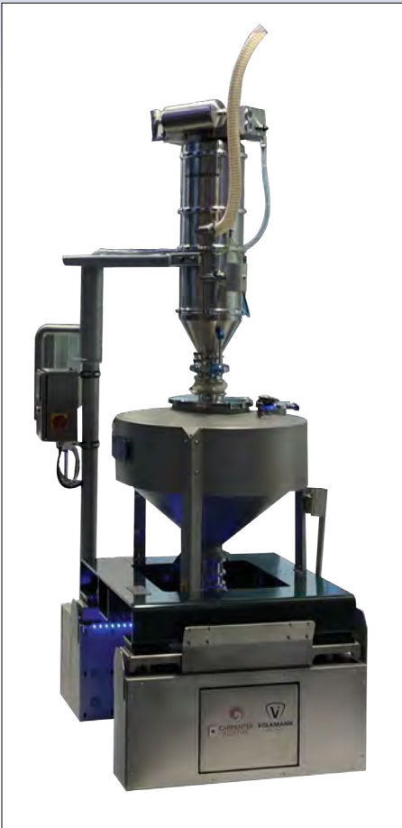
Fig 6: Recently displayed at FormNext is a 130-l IBC on a docking and weighing station along with a conveyor used for refilling the IBC with material that has been screened after passing through the printer build box.
