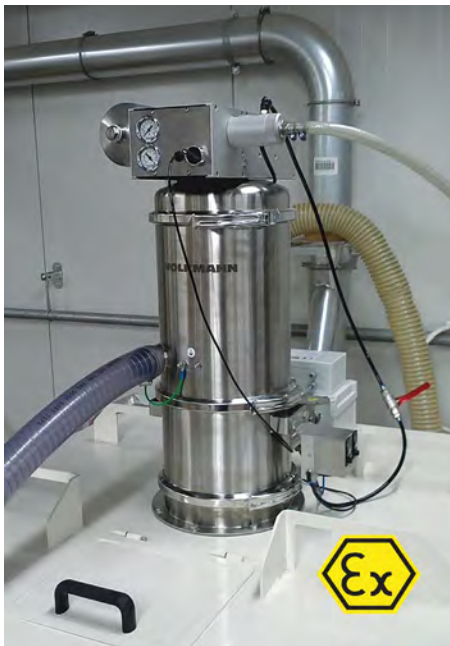
ATEX-certified pneumatic vacuum conveying systems permit safe material transfer in explosive environments. Volkmann VS Series model 250 is shown.
