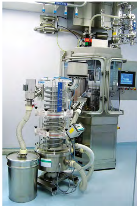
An INEX pneumatic vacuum conveying system from Volkmann automatically transfers powders to a tablet press under an inert atmosphere. This system earned ATEX certification by eliminating the potential for ignition and avoiding explosions.
