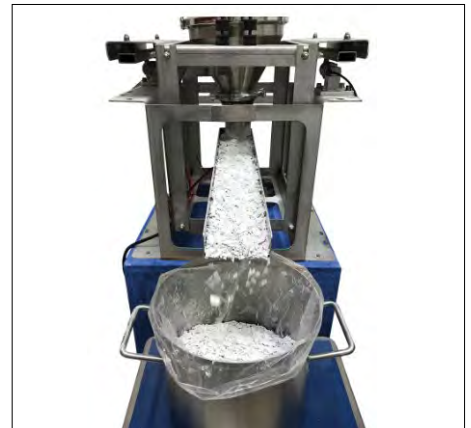
This vibratory weigh feeder from Volkman features an optional, built-in load cell for weighing. It automatically weighs a preset amount of material and gently advances it either continuously or in precise doses.
