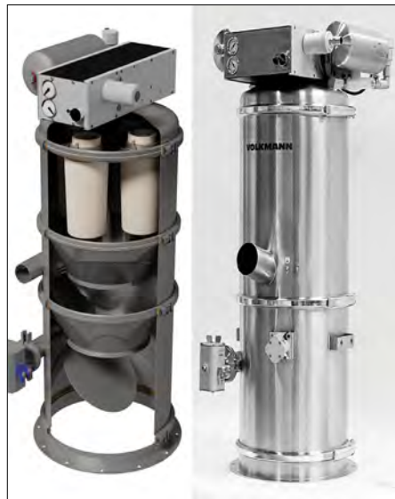
Access for cleaning and inspection is critical for smooth changeovers. The Volkmann VS vacuum conveyor shown earned a patent for quick disassembly without tools for access to the filter system inside.
