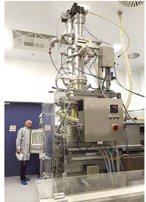
A plant engineer watches as a pneumatic vacuum conveying system from Volkman automatically transfers powder up and into a stick pack machine. Transferring finished products up and into filling and packaging lines automatically speeds production, prevents contamination, and promotes a clean, sanitary work environment (Volkman USA).
