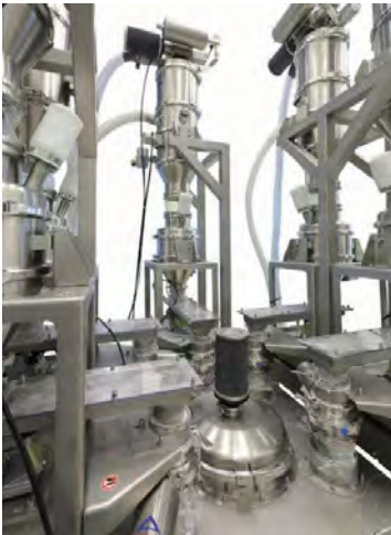
Pneumatic vacuum conveyors from Volkman transfer multiple materials from multiple locations then companion vibratory weigh feeders weigh and dose them into a central tank. The entire process may be automated as shown or the weighing and feeding functions alone may be automated.
