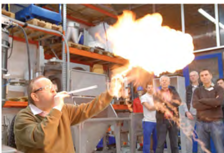
Fig 2. Metal powders are also known to be explosive; some are even selfigniting in certain conditions.
