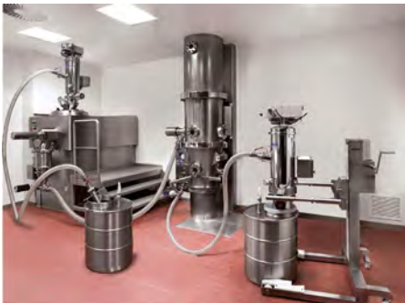
Figure 2: Volkman-VS-Conveying: The latest pneumatic vacuum conveying systems like this ATEX-certified Volkman VS Series model 250 eliminate the potential for an explosion rather than suppress, contain, or vent the explosion after the fact.
