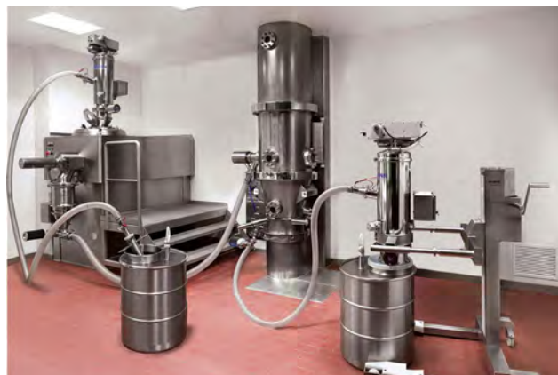
Pneumatic vacuum conveying systems like the one shown in stainless steel from Volkmann are often used to transfer multiple materials and ingredients from different pickup points due to their designed-in cleanability for fast changeovers.
