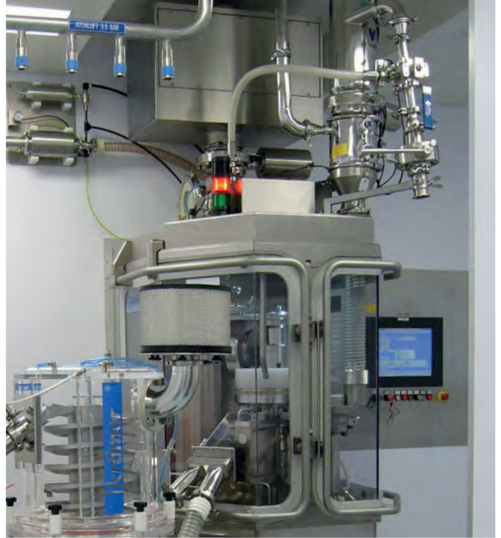
PPC (WIP) for charging a tablet press.
