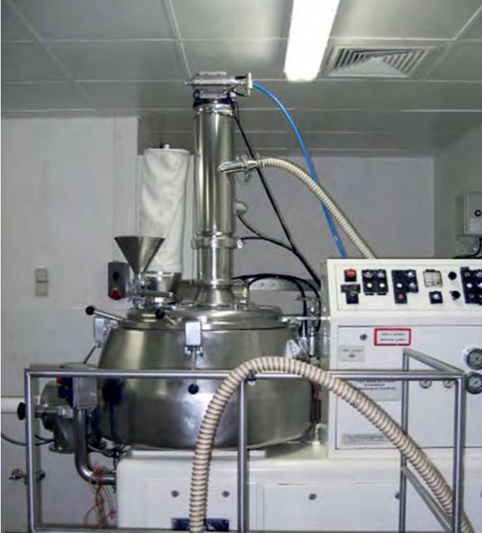
Loading of the mixer using PPC.
