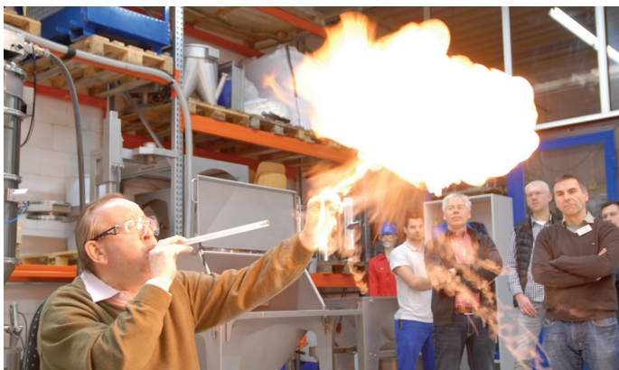
Swiss expert Dr. Glor demonstrating that "the long duration of the flame compared to a gas explosion makes dust explosions particularly dangerous" during a recent seminar at a leading vacuum conveyor company seminar in Soest, Germany.
