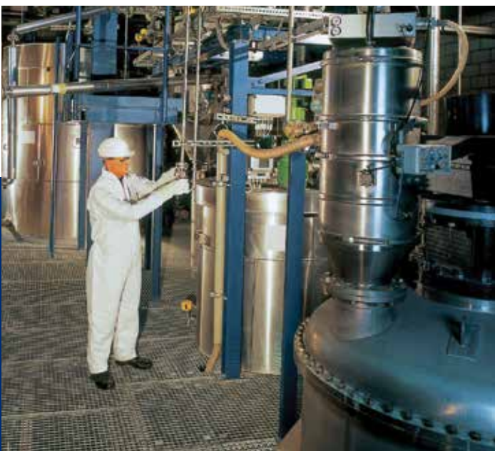
Figure 3: Vacuum conveyor (front, right) for the feeding of powders into a process vessel (beneath)
