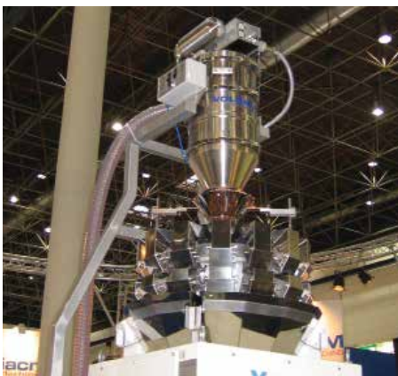
Loading of a multiple-bucket-weighing and dosing system.
