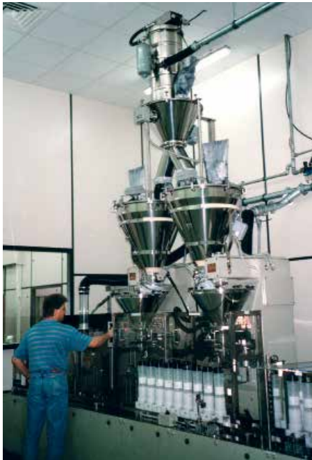
Carbon black toner transferred via a Volkmann conveyor to a bottle filling machine.
