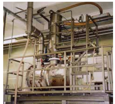
Vacuum Transport and loading of a mixer with powders for sauce-making.
