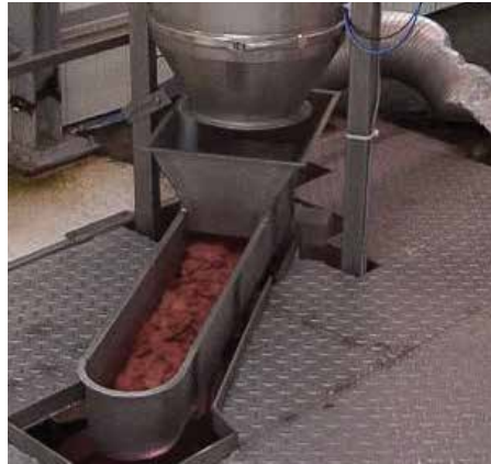
Transport of salami-slices for pizza-topping.
