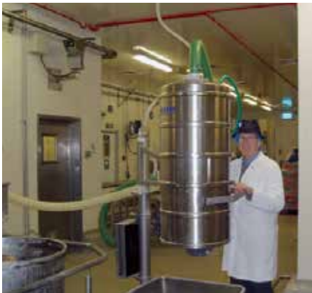
Flour transfer system in a bakery.
