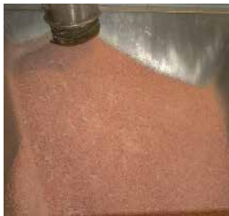
Granulated meat conveying in sausages-making process.
