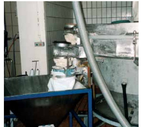
Feeding from a tumbling-sieve into a hopper for Vacuum Transfer.
