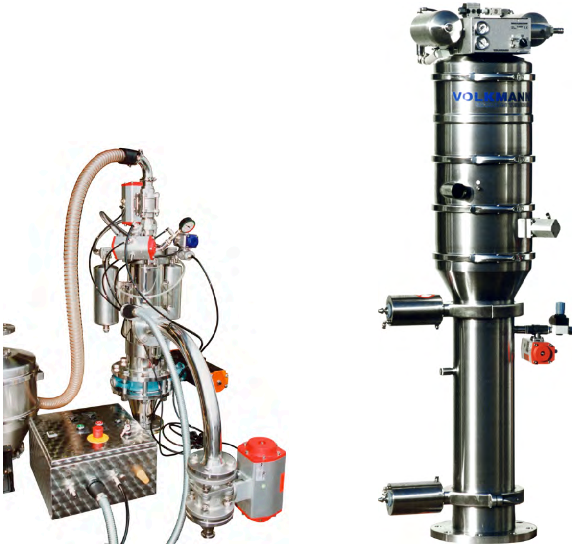
Fig 3 – Examples of an Inert Gas Based Conveyor (Left) and a Powder Lock System (Right)
