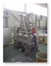
Figure 2: Two Vacuum Conveyors transfer different powders onto a powder processing/ production line; for the conveying pipeline here hoses were chosen.
