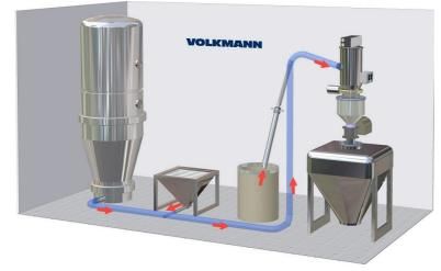
Figure 1: Exemplary layout of a Volkmann vacuum conveying system including three different pick-up points, conveying line, conveyor and the material's destination. (A container is shown.)
