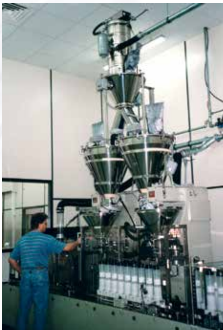
Carbon black toner transferred via a Volkman conveyor to a bottle filling machine.
