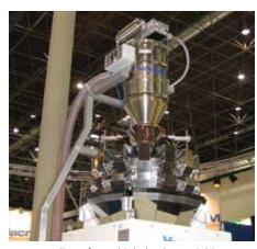
Loading of a multiple-bucket-weighing and dosing system.
