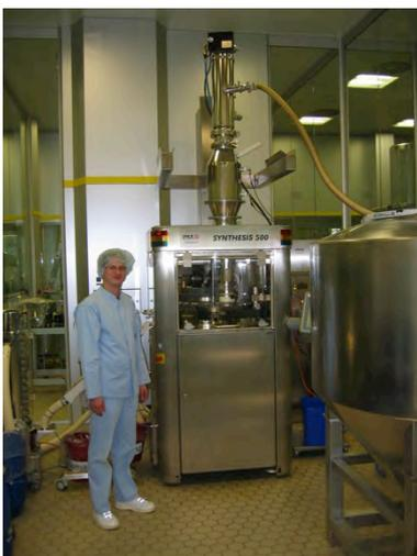
Feeding of pharmaceutical powder into a tablet press with a Volkmann Vacuum Conveyor (shown on top of the tablet press)
