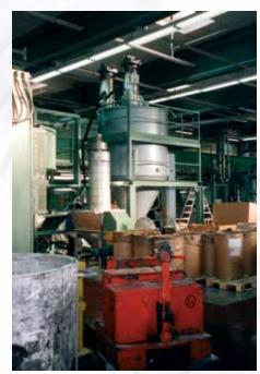
Carbon black toner transferred via a Volkmann conveyor to a bottle filling machine.
