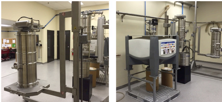
Left to right; VS350 on variable adjustable mobile frame and IBC Filling and Unloading station. Conveying lines are visible along the walls.
