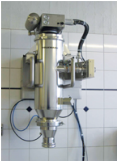
Volkmann PPC in the weigh frame of a dosing process. Conweigh element at rear of PPC.
