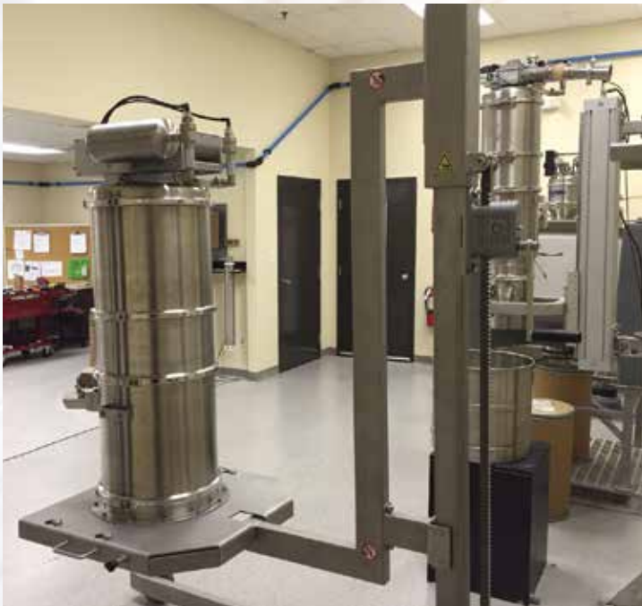
Left to right; VS350 on variable adjustable mobile frame and IBC Filling and Unloading station.
