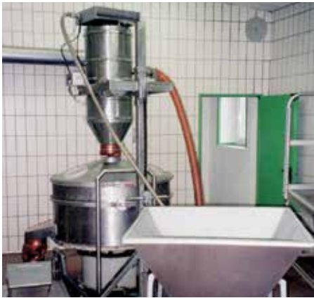
Conveying of spices from a hopper and loading of a sieve.
