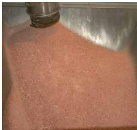
Granulated meat conveying in sausages-making process.
