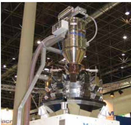
Loading of a multiple-bucket-weighing and dosing system.
