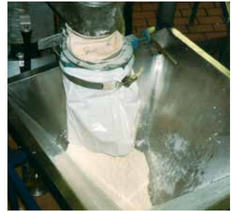
Loading of Cream-Fat powder (70 % fat) into a hopper and filling Big-Bags.
