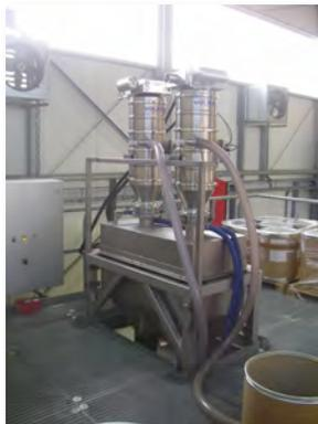
Figure 2: Two Vacuum Conveyors transfer different powders onto a powder processing/production line; for the conveying pipeline here hoses were chosen.
