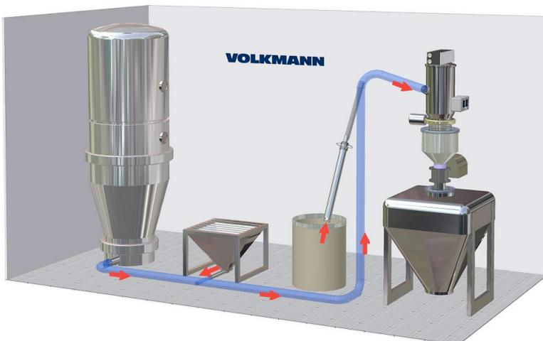
the vacuum through a suction hose or pipe into the bulk material receiver. From there the material drops into its destination point (**Figure 1**). The result is an active, dust-tight feeding from the top without positive pressure. Following this principle, a variety of bins, big-bags and processes are able to be supplied with powders and bulk materials.
