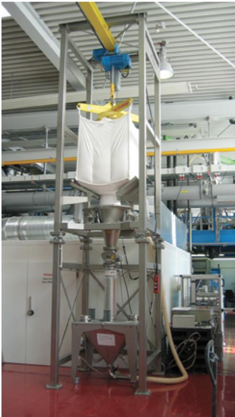
Hoist style BBU with special loss-in-weight features.
