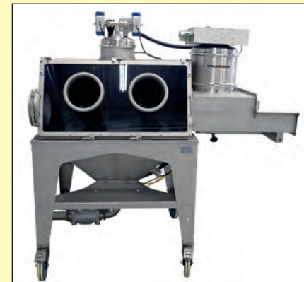
Glove box and filtered bag dump station
