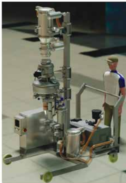
Inert harvesting station
