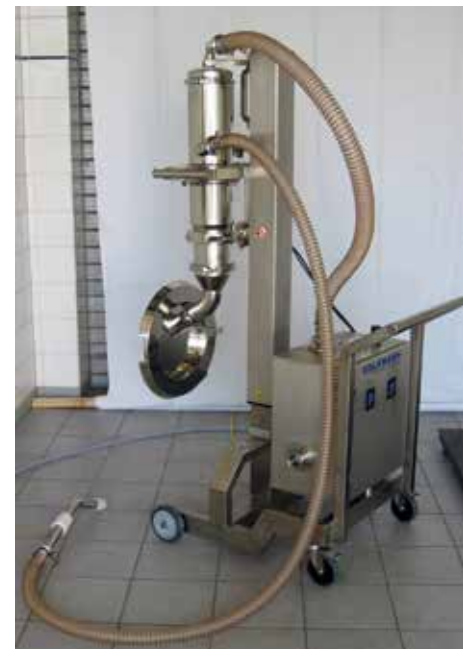
Mobile hoist with filter and suction hose.
