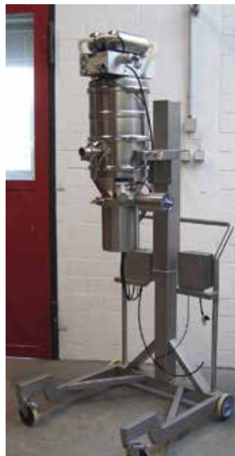
Mobile hoist with control box mounted on top.
